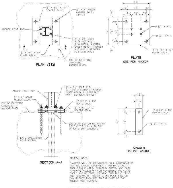
RETROFIT SLIP BASE PLATE DETAIL FOR GUARD CABLE ANCHOR POST REPAIR
