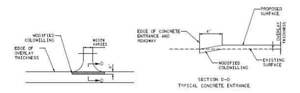
**2.7** The bituminous pavement shall be coldmilled and tapered at the Railroad (see pavement taper details below).
