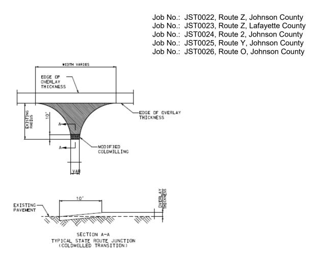
**2.5** The bituminous pavement shall be coldmilled and tapered at entrances and non-state routes (see pavement taper details below).
