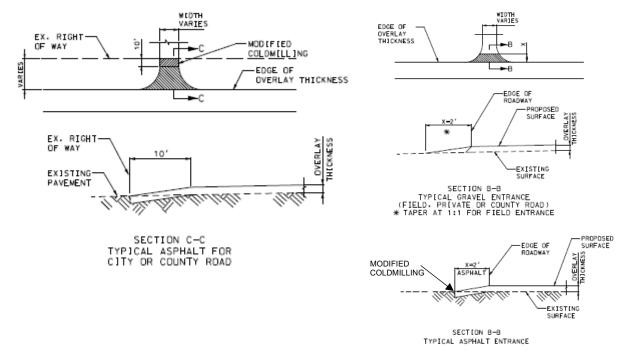
**2.6** The bituminous pavement shall be edge coldmill for concrete entrances or non-state routes (see pavement taper details below).
