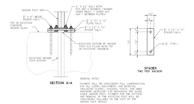
RETROFIT SLIP BASE PLATE DETAIL FOR GUARD CABLE ANCHOR POST REPAIR
