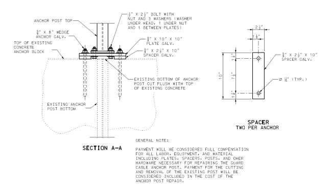
RETROFIT SLIP BASE PLATE DETAIL FOR GUARD CABLE ANCHOR POST REPAIR
