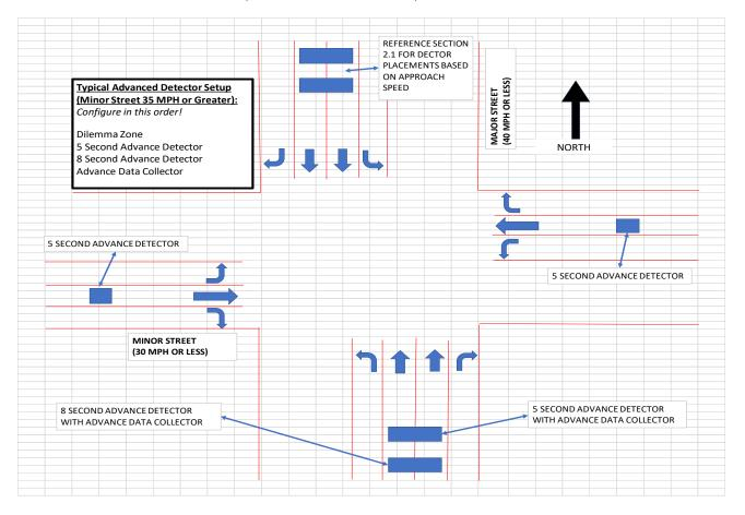
**2.1 Detector Zones.** Advanced detection zones shall be placed at 5 seconds and 8 seconds travel time before stop bar per below Table unless directed otherwise in the plans or by the Engineer. If curvature of the road or obstructions prevent tracking of vehicles, priority should be given to detection at the 5 second and 8 second distances.
