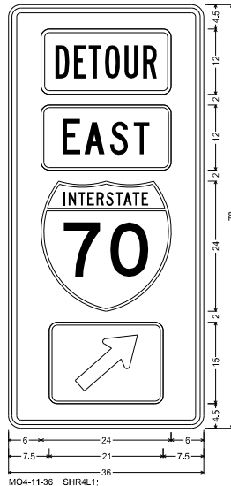
MO4-11-36 SHR4L1: 2,250" Radius, 0.875" Border, 0.625" Indent, Black on Orange; Table of letter and object lefts.
