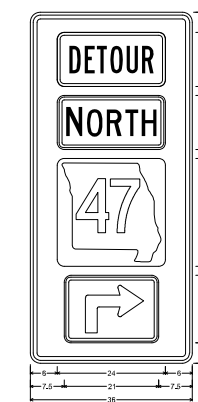
MO4-11 SHIF-FLAT SHEET FLUORESCENT: 2.250" Radius, 0.875" Border, 0.625" Inset, Black on, Orange Table of letter and object belts 1 0.500 2 1.000 3 1.500 4 2.000 5 2.500
