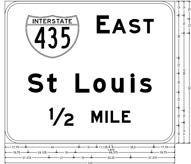
E1-1 ST-STRUCTURAL: 12,000" Radius, 2,000" Border, White on, Green; Interstate 435 18,000" B; "EAST", E Mod; "St Louis", E Mod; "1/2", E Mod; "MILE", E Mod; Table of letter and object lefts
