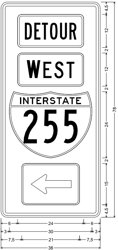
MO4-11-36 SHF-FLAT SHEET FLUORESCENT; 2.250" Radius, 0.875" Border, 0.625" Indent, Black on, Orange; Interstate 255 12.000" B;
