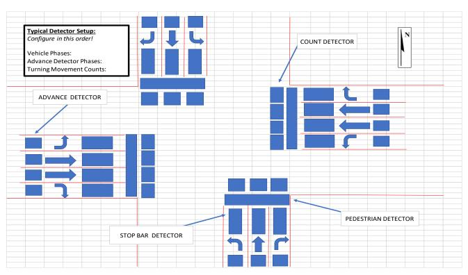
Dilemma zone detectors shall be placed at 5 secs and 8 seconds travel time before stop bar per below Table unless directed otherwise in the plans or by the Engineer.
