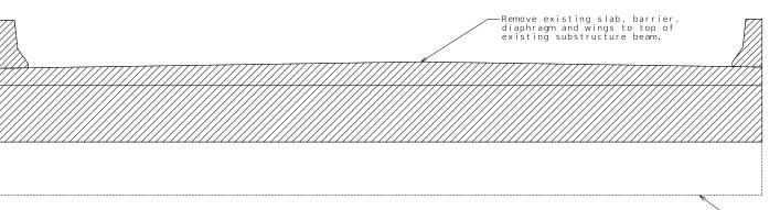
DETAILS OF CONCRETE REMOVAL AT END BENTS
