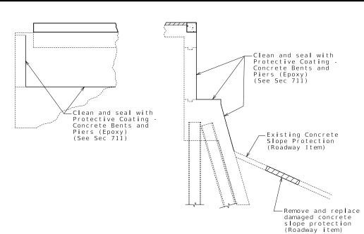
TYPICAL SECTION THRU ABUTMENTS NO. 1 & 3 SHOWING PROTECTIVE COATING AND REPAIR OF CONCRETE SLOPE PROTECTION
