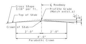
TYPICAL SECTION THRU SLAB
