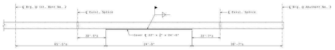
PART ELEVATION OF INTERIOR GIRDER SHOWING COVER PLATE INSTALLATION SPAN (2-3)
