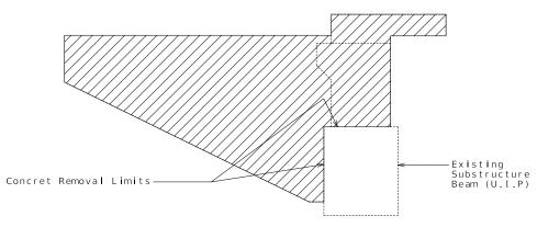
PART SECTION SHOWING CONCRETE REMOVAL AT END BENTS
