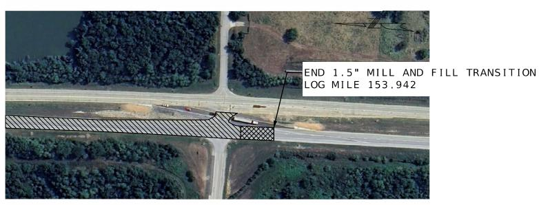
1.5" MILL AND FILL FROM BEGINNING OF CONCRETE BARRIER TO S/O SE 700 RD MATCH NB CONCRETE PAVEMENT LOG MILE 151.901 TO LOG MILE 153.942 EXCEPT BRIDGES
