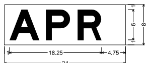
SHF-FLAT SHEET FLUORESCENT; No border, Black on Orange; [APR] E Mod; Table of letter and object lefts.
