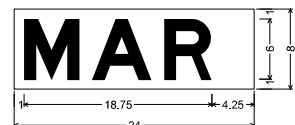
SHF-FLAT SHEET FLUORESCENT; No border, Black on Orange; [MAR] E Mod; Table of letter and object lefts.
