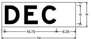
SHF-FLAT SHEET FLUORESCENT; No border, Black on Orange; [DEC] E Mod; Table of letter and object lefts.
