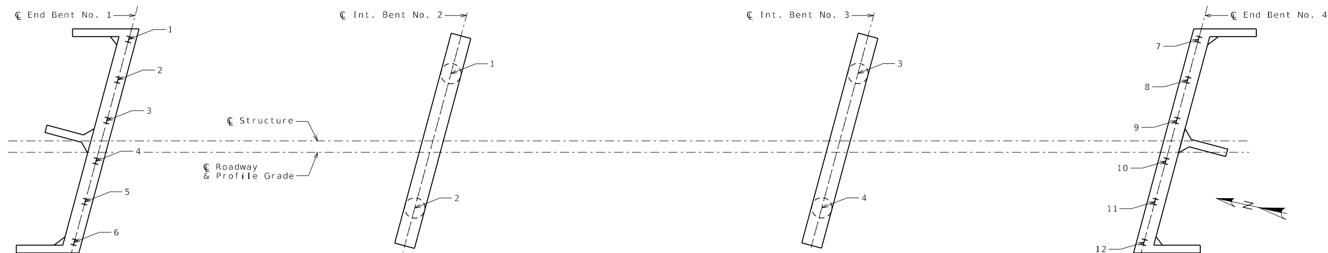
PART PLAN SHOWING PILE & DRILLED SHAFT NUMBERING FOR RECORDING AS-BUILT PILE DATA & AS-BUILT DRILLED SHAFT DATA
