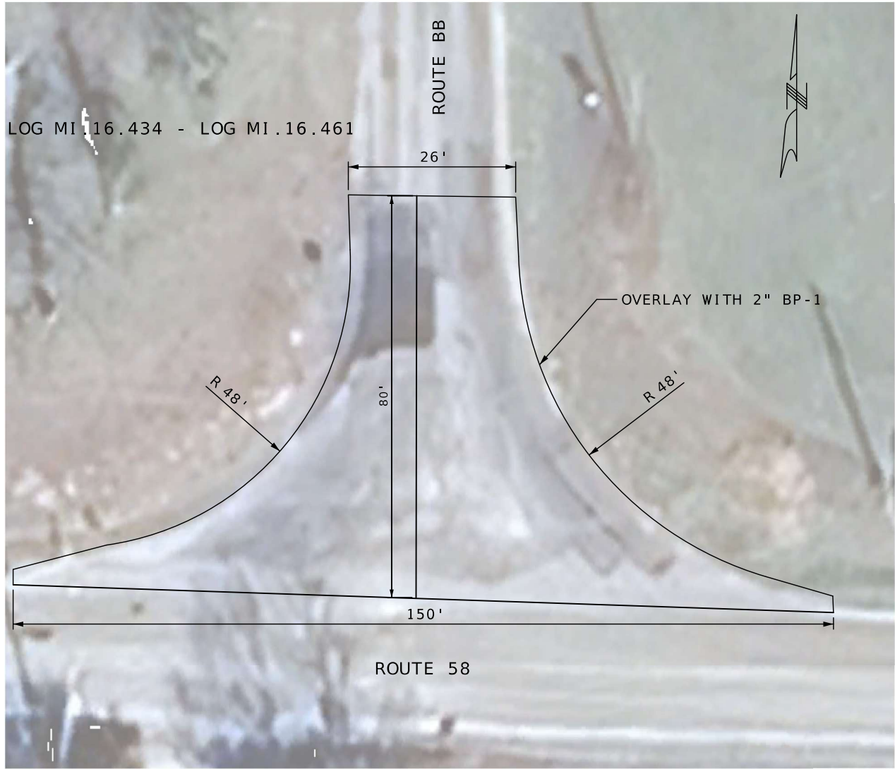
LIMITS OF PAVING ROUTE BB
