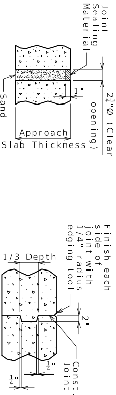
UNDERSEAL ACCESS HOLE DETAIL
